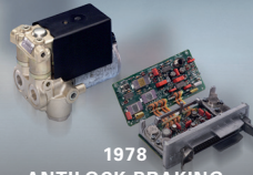
1978 ANTILOCK BRAKING SYSTEM (ABS) by Bosch
